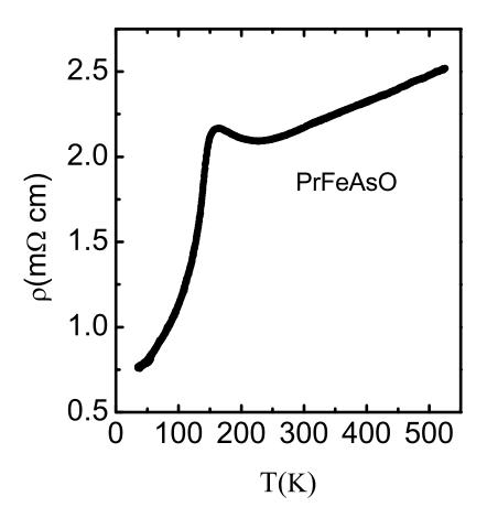
FIG. 3: Temperature dependence of resistivity for the nonsuperconducting PrFeAsO sample.
