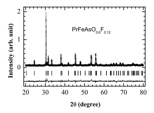
FIG. 1: The x-ray diffraction pattern for the superconducting PrFeAsO<sub>0.6</sub>F<sub>0.12</sub> sample. The solid line corresponds to Rietveld refinement of the diffraction pattern with P4/nmm space group.
